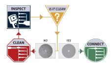
Contamination is the number 1 reason for troubleshooting optical networks. Proactive inspection and cleaning of fiber connectors can prevent poor signal performance, equipment damage, and network downtime.
